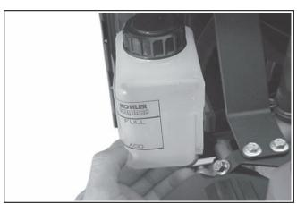
Figure 13. Removing Reservoir.
